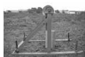
Roller must be completely stable.
